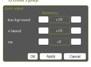
the sorting process, the algorithm autonomously decides which products are removed. If your operators still detect errors, they can easily adjust the algorithm by classifying extra object images or via "Quick adjust".
