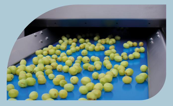
Picking grapes, dates and cherry tomatoes with the destemmer surpasses manual processing. The machine is unique because, like no other comparable machine, it can pick the fruit from the vine with a rotating movement. Which is just how it would happen if picked by hand. The point where the stem meets the fruit thus remains intact, improving shelf life.
