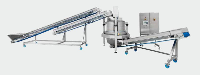
The K650 drying system is the ideal system for drying a wide variety of lettuce and vegetable products in a continuous treatment process. The K650 drying system is perfectly suited for drying sliced fruit, vegetables, lettuce, mushrooms and herbs in the industrial application.
