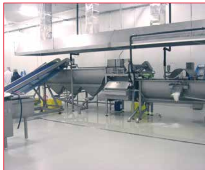
Turkey: Large salad processing line – capacity up to 1.500 kg/h
